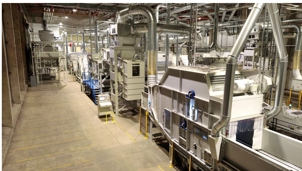
ANDRITZ hemp decortication line in operation at Ekolution
